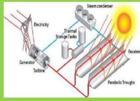
Two main types: Central Receiver and Parabolic Trough. Water, or another working fluid is heated by concentrating sunlight on a receiver. Usually steam is created then expanded through turbine to generate electricity. Most solar power plants have some kind of storage system where hot fluids can be kept hot for later use (when the grid needs electricity).
